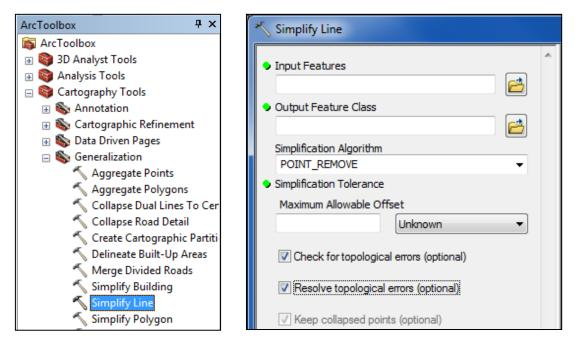
These parameters are appropriate in most cases for medium scale (EBM/ERM). Alternatively, the following parameters might be used:
